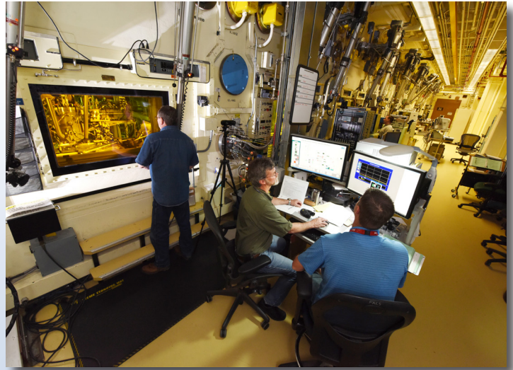
The main hot cell is 70 by 30 feet with 15 workstations each at a 4-foot-thick window.
